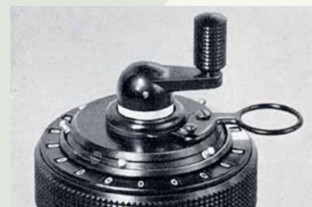
**Lifting the crank for subtraction**
